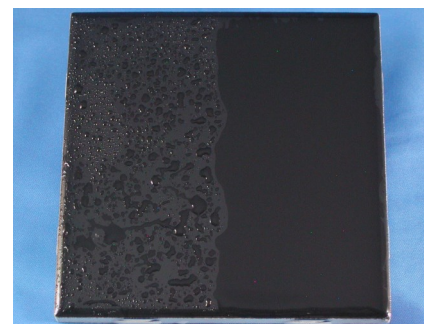
Figure 2: Right half of tile treated with 0.5% Flexipel SR-80 exhibits complete hydrophilization.
