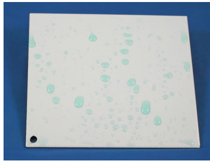
Figure 1: Untreated panel exhibits hydrophobic nature.
